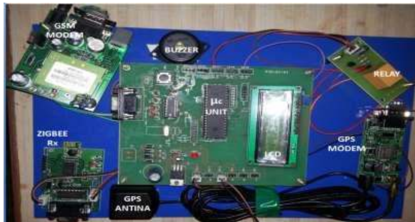
Figure-8: Main Controller Unit
