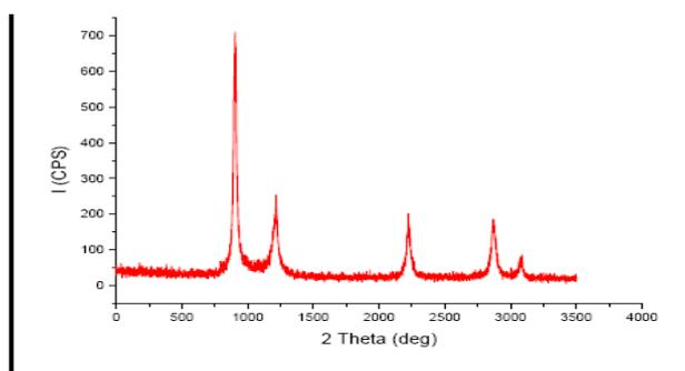
Figure 1: Typical XRD pattern of silver nanoparticles synthesized using leaf extract of *Semecarpus anacardium* Linn.F.
