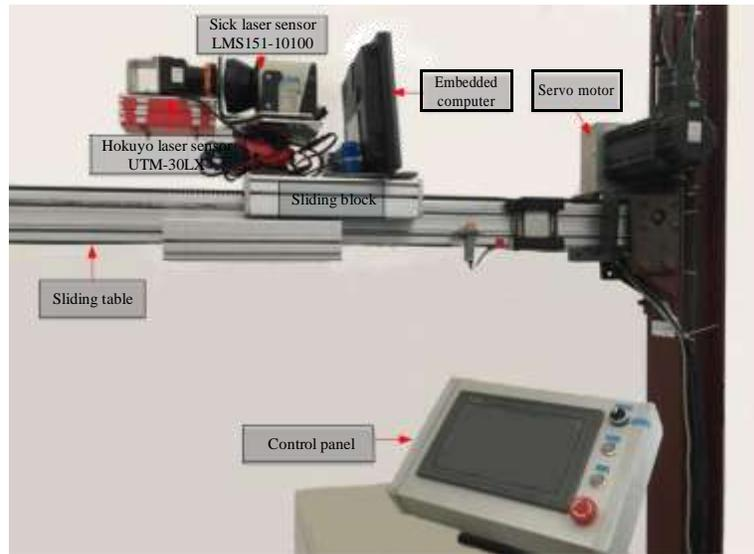
**Figure 4** Lidar-based indoor target detection system
