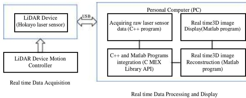
**Figure 1.** Real time data acquisition and data processing scheme.
