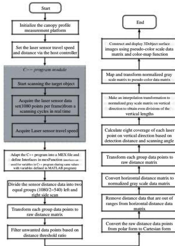
**Figure 3** Flow chart for the MATLAB algorithm program compiled with the C++ program module for detecting and constructing 3-dimensional object surfaces.
