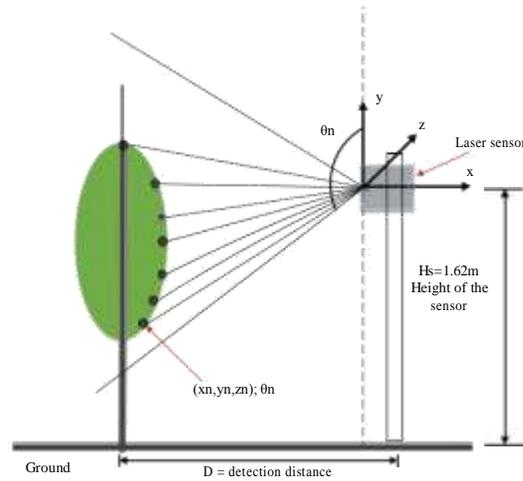
**Figure 2** Operational principles of the laser sensor: Each laser beam return is characterized by the distance and angle referred to  $0^\circ$  of the position of the laser sensor.
