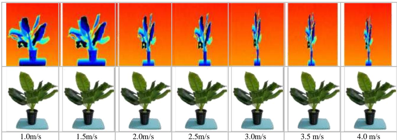
**Figure 6.** Paired images of the artificial tree-1 obtained from the digital camera and the laser sensor. The pseudo color images from the laser sensor were reconstructed in real time from the dataset acquired at 2.0 m detection distance and various laser sensor travel speed (1.0, 1.5, 2.0, 2.5, 3.0, 3.5 and 4.0 m/s).
