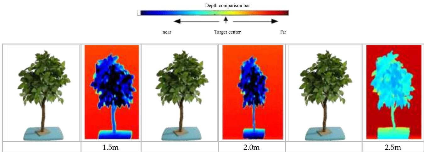
**Figure 7.** Paired Images of the artificial tree-2 obtained from the digital camera and the laser sensor. The pseudo color images were reconstructed from the sensor raw data obtained at 2m/s sensor travel speed and different target detection distances(1.5,2.0 and 2.5m) in real time.
