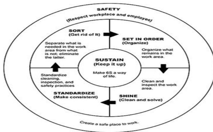
*Figure 1.* – 6S Flow Diagram<sup>26</sup>
